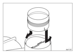
If using 5" (125 mm) ducting, place the reducing collars into the exhaust connections and turn left to lock them in place.
